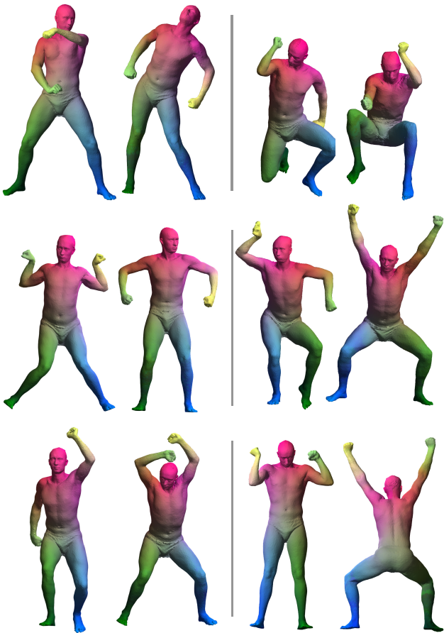
Figure 7: Examples of typical maps obtained with PM-SDP on the SCAPE dataset [Anguelov et al., 2005]. In all pairs: left mesh is colored using a predefined color map; right mesh is colored according to the correspondence. Bottom right: a failure case.
